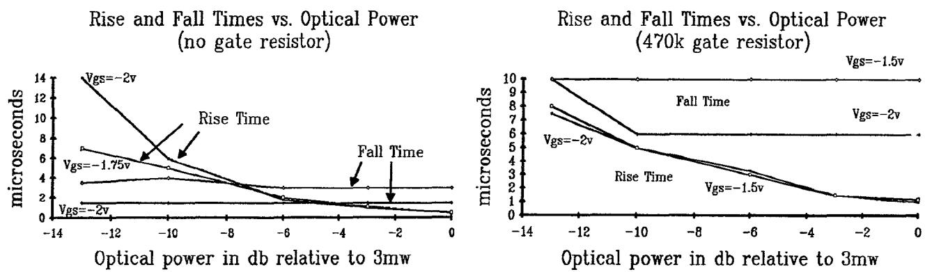
Fig. 2 Rise and fall times for the FUJITSU MESFET operated under pulsed illumination (a) without gate resistor (b) with a 470k gate resistor.
