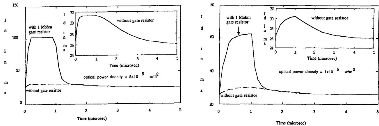
Fig. 1 Drain current optical pulse response of the MESFET (solid line - total, dashed line and insert - internal). optical power density = (a)  $5 \times 10^5 \text{ w/m}^2$  (b)  $1 \times 10^5 \text{ w/m}^2$
